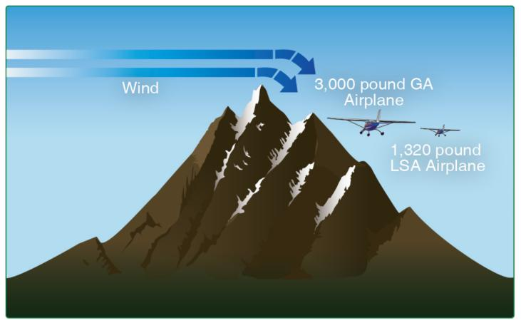
Figure 17-7. Moderate mountain winds can create severe turbulence for LSA.
