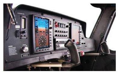
Figure 17-11. Stoke flight control with conventional engine controls.
