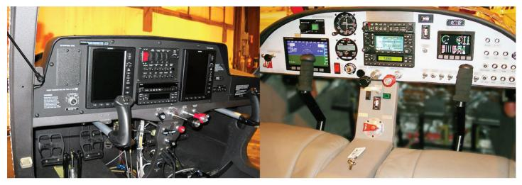
**Figure 17-5.** An electronic flight instrumentation system provides attitude, airspeed, altimeter, vertical speed, direction, moving map, navigation, terrain awareness, traffic, weather, and engine data all on one or two liquid crystal displays.
