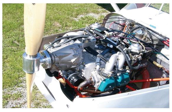
Figure 17-4. A water-cooled 4-cycle engine.
