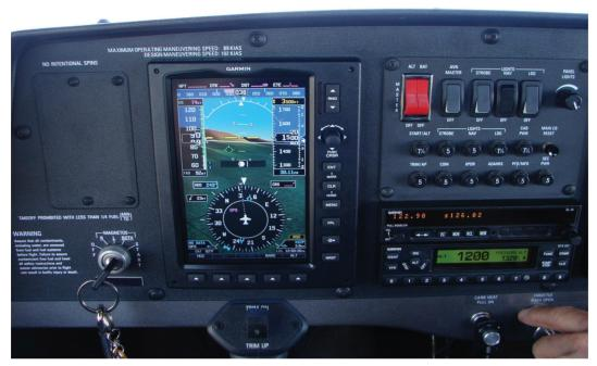
Figure 17-15. EFIS indication of level cruise flight.
