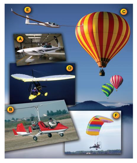
**Figure 17-1.** The LSA category covers a wide variety of aircraft including: A) airplane, B) gyroplane, C) lighter-than-air, D) weight-shift-control, E) glider, and F) powered parachute.
